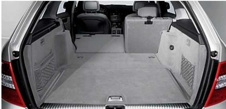
The load compartment has a capacity of up to 1500 litres with the rear seat backrest folded
