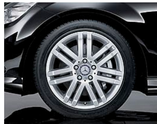
17-inch 7-twin-spoke light-alloy wheel
